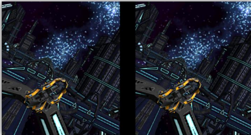
Fig. 3 The SDK is splitting and distorting the original image in two so that there are two images (one for each eye) in order to create a 3D effect [8]
