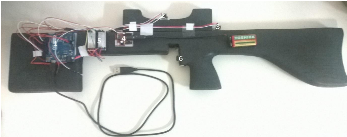
Fig.1 1.Arduino board, 2.IUM sensor, 3.Proximity sensor, 4.Power supply, 5.Breadboard (for wire connecting ), 6.Button A
