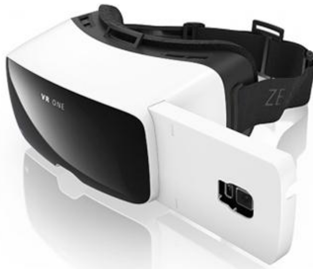
Fig. 2 VR One headset with its tray in which the smartphone is introduced [7]
